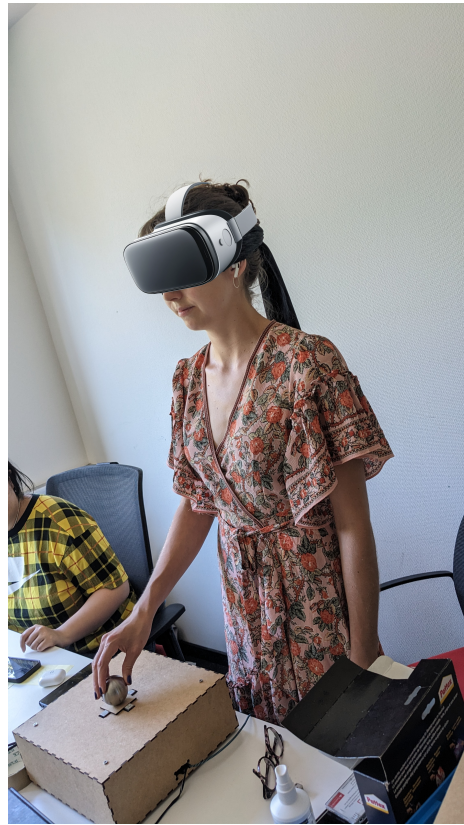
Fig. 2. The participant will be wearing a VR headset while feeling the motion illusion in VR. The kinesthetic display is connected to the computer.
