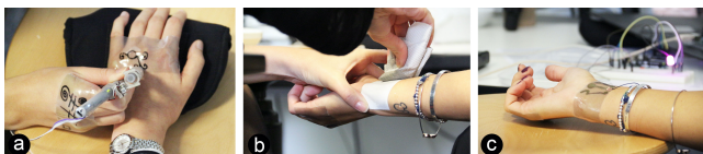
Figure 15: Artists during focus group exploration. Inking on each-other (a), applying substrate for functional prototype interface (b), completed epidermal interface controlling an RGB LED (c).
