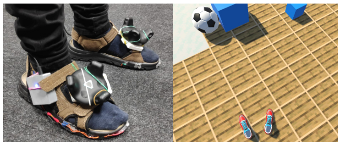
Figure 5. bARefoot prototypes augmented with HTC Vive sensors to track the positions of the user’s feet (left). First-person view of the VR application within which the user can experience walking on various virtual materials.
