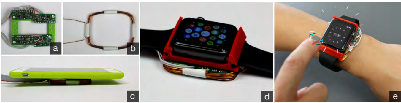
Figure 1: Magnetips consists of (a) a magnetometer array to track the magnet on the fingernail, and (b) a coil to provide haptic feedback to it. These can be used simultaneously and integrated with mobile devices (c,d) to enable interactions in the space around the watch (e).
