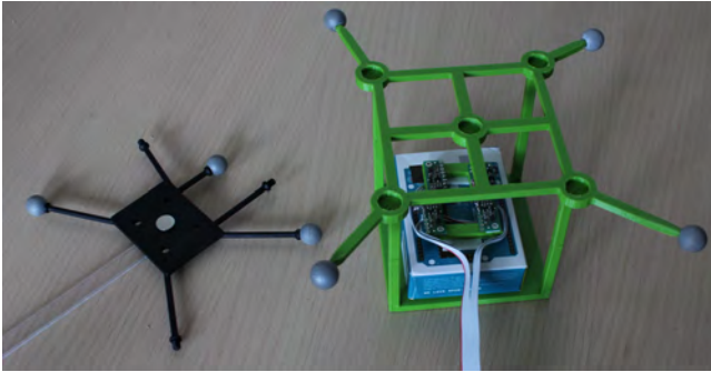
Figure 3: A setup of how the magnet and sensor board was tracked using OptiTrack.
