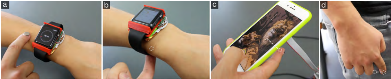
Figure 8: Magnetips enables these interactions: a) 3D mid-air, b) Behind arm, c) Back of device, d) Through material.
